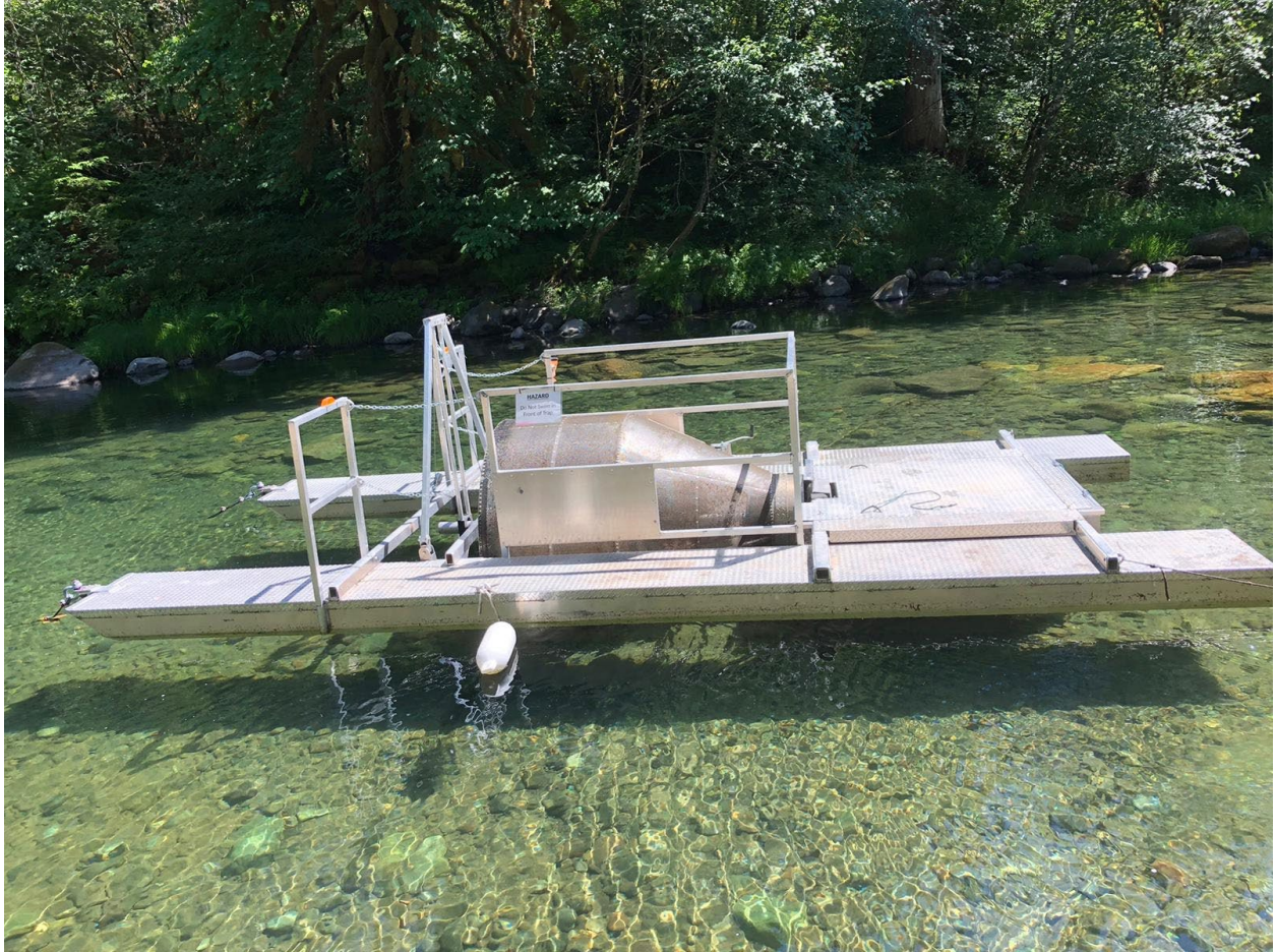
Figure F-4. RST sampling at the Green Peter Head of Reservoir – Middle Santiam site in low flow.
