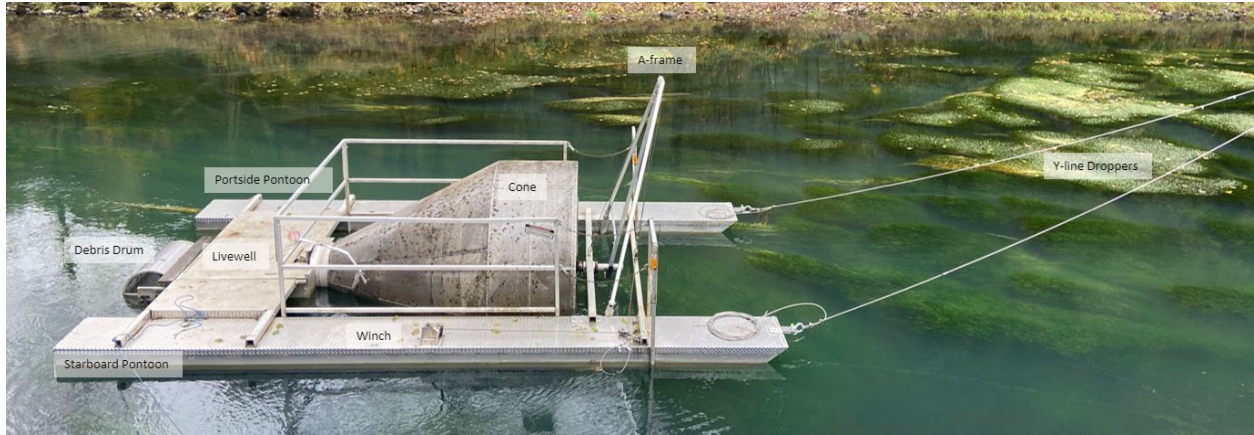
Figure F-1. Labelled image of a rotary screw trap showing parts and terminology.
